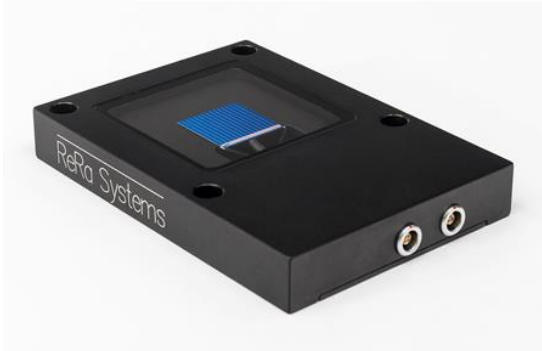
The reference Si cell has active area of 2 x 2 cm
