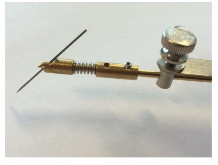
**Optional: 2-pin BeCu probe tip (required for 4 point measurements)**
